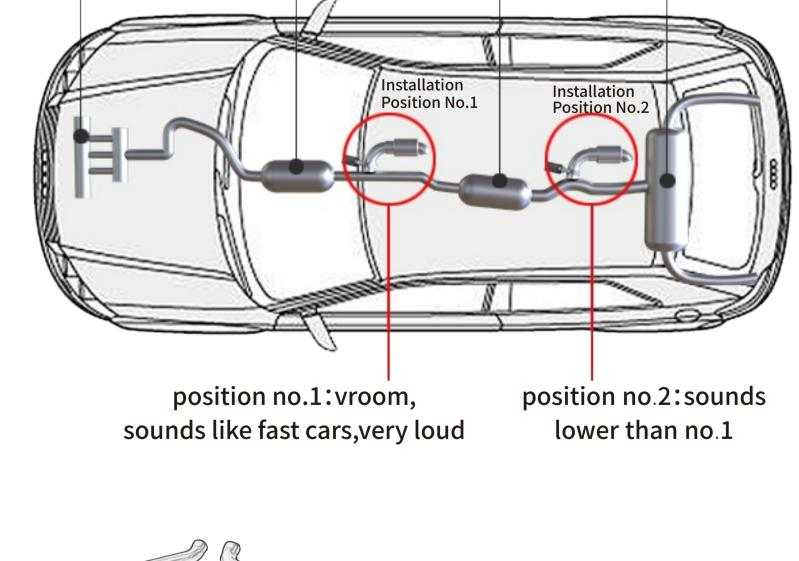
Catalytic Converter Middle Muffler Rear Muffler
